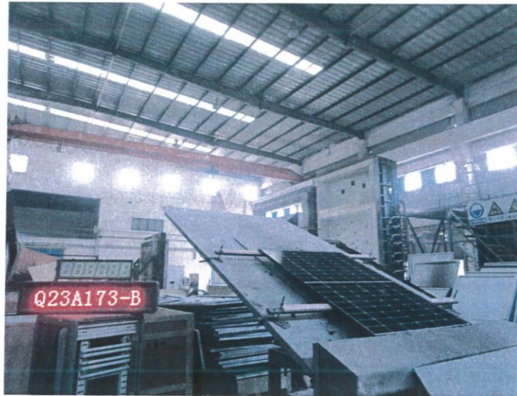
Figure 3: Photovoltaic panel before Burning-Brand Test Q23A173-B
