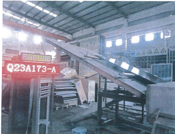
Figure 1: Spread-of-Flame test set-up for Q23A173-A
