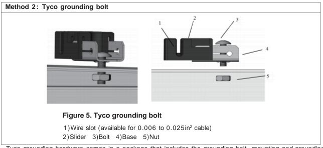
Tyco grounding hardware comes in a package that includes the grounding bolt, mounting and grounding hex nut.
