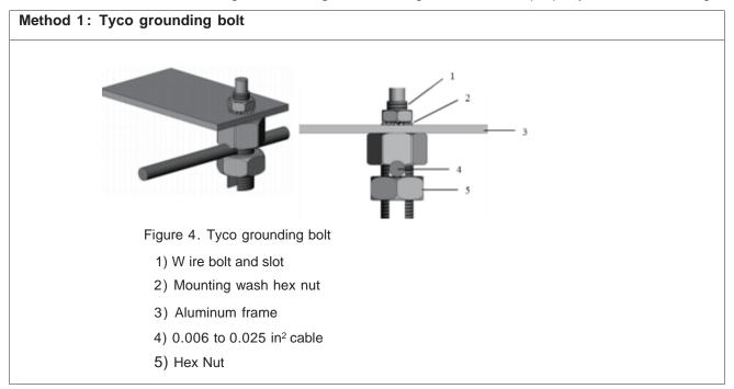
Tyco grounding hardware comes in a package that includes the grounding bolt, mounting and grounding hex nut.
