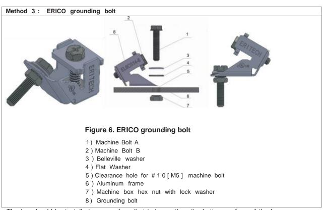
The lug should be installed on a surface that is larger than the bottom surface of the lug.
